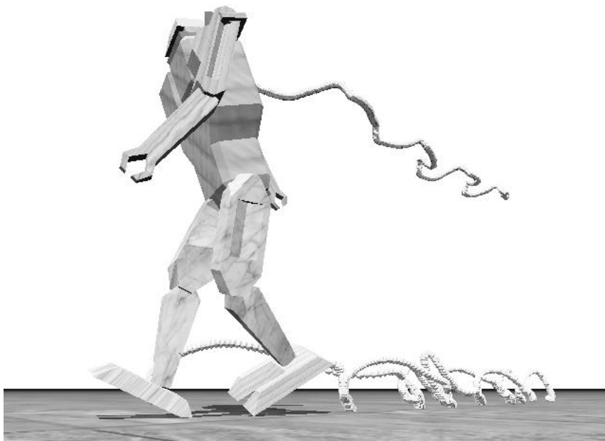
Figure 7.14: Biped walking, without hip side compensation. The biped sways from side to side as it walks (the trail left by the head has a large side-to-side variation).
